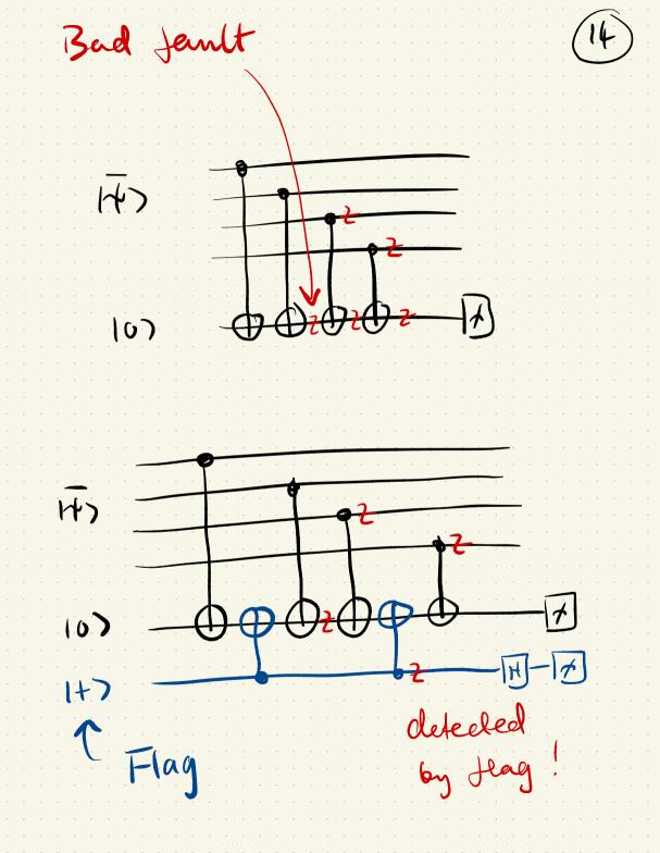
In general, for Henry EC (15) we only need 2 extra Hay qubits for femilt tourant stabilizer measurement. Aside: In the (20) surface code, these construction are not necessary & familt tolerance cen be actieved by repeating the stabilizer measurements O(d) they where d is the code distance.
